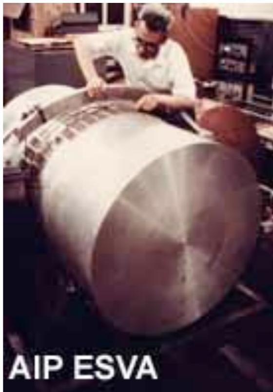
Resonant bar detectors: very narrow band and limited sensitivity
